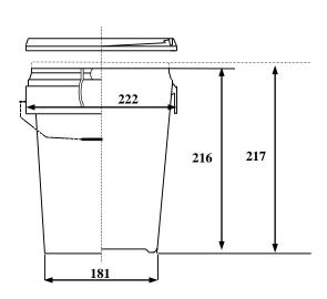
Measurements in millimetres
